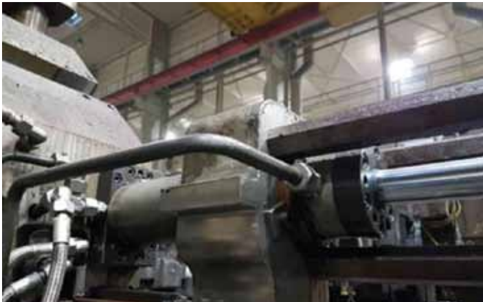
ZAF - ROUND-CYLINDER WITH PLASMA-NITRATED BODY USED AS A GUIDE
