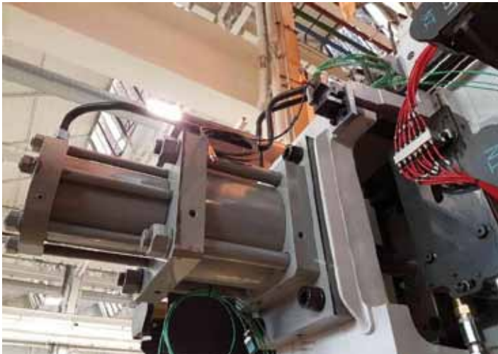
ZAF - ROUND-CYLINDER WITH PLASMA-NITRATED BODY USED AS A GUIDE
