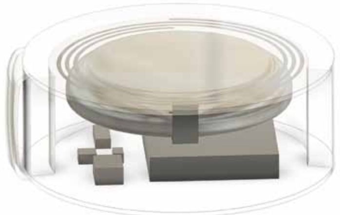
Miniaturized sensor package after folding the substrate over the frame
